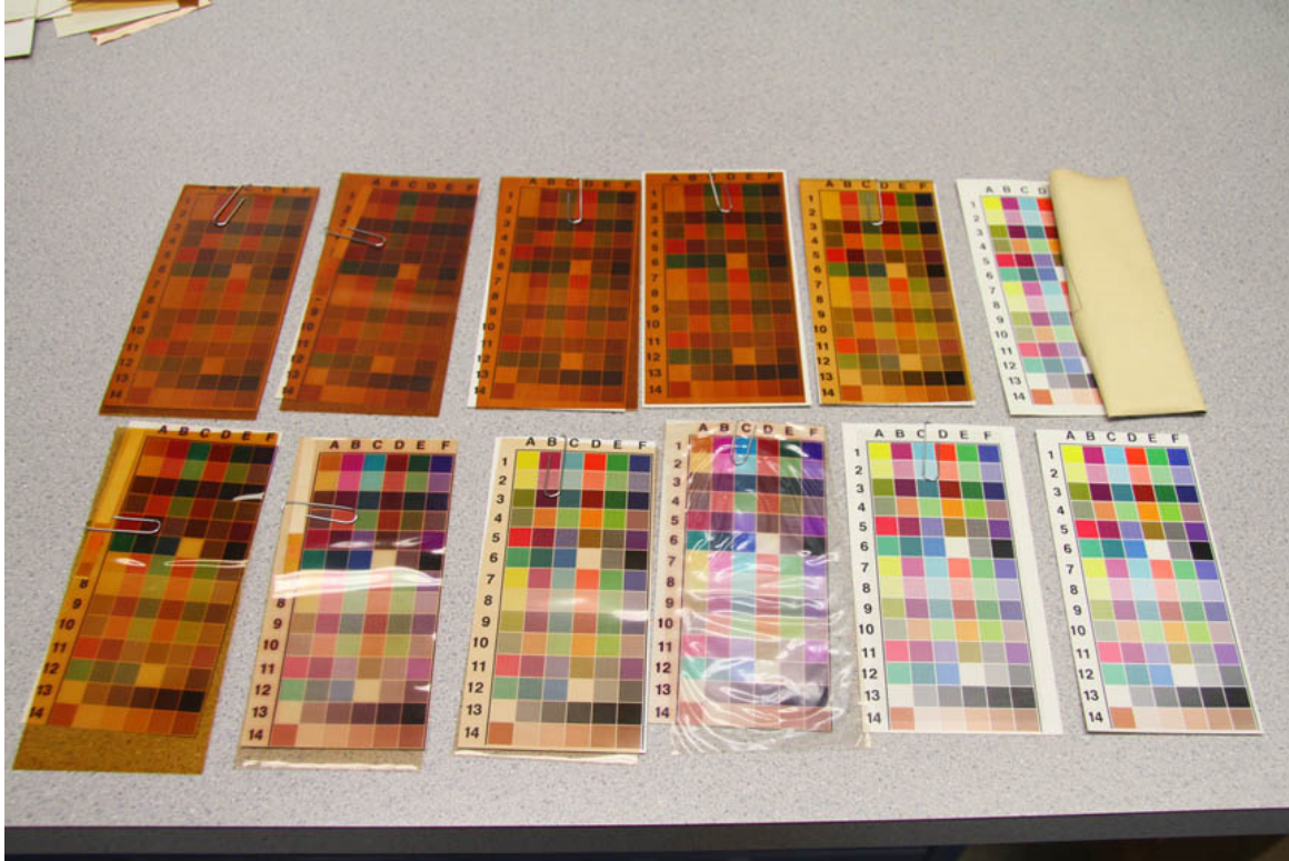
Figure 4 – Degradation of PVC samples after seven weeks at 85C/50%RH
