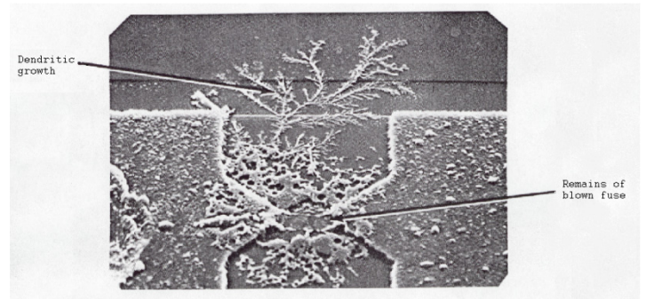
Figure 6. Dendrite growing out of remains of blown fuse. 15
