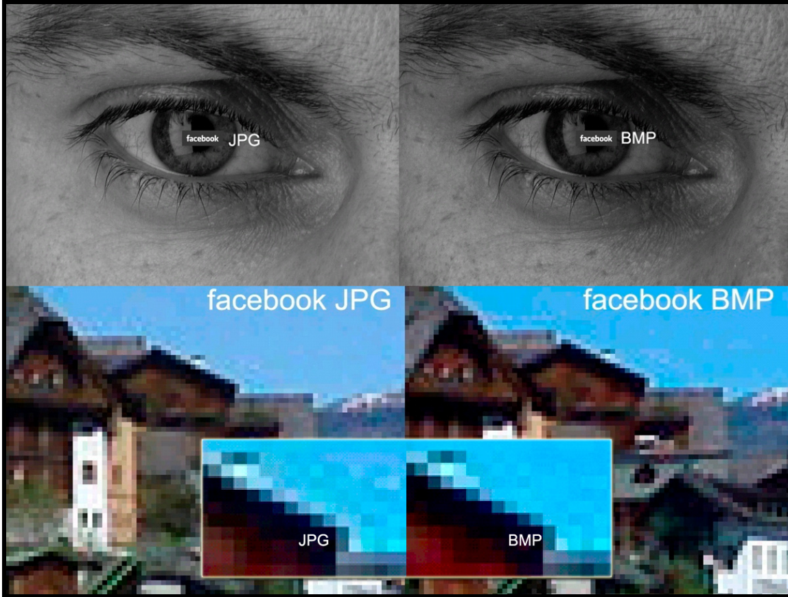
Figure 3. Facebook JPG & BMP downloads demonstrating reduced BMP color depth even in B&W, no detail loss due to JPEG Blocking:
