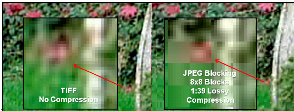
Figure 2. Two camera image captures; one as a TIFF with no compression and as a high compression JPEG demonstrating JPEG Blocking:
