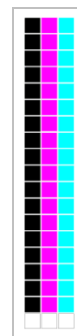
Fig. 4: Test target. (57 blocks, neutral d_{max} on left, magenta center, cyan on right, neutral d_{min} on bottom)
