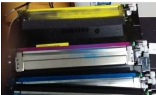
Figure 1. Toner leakage at development unit
