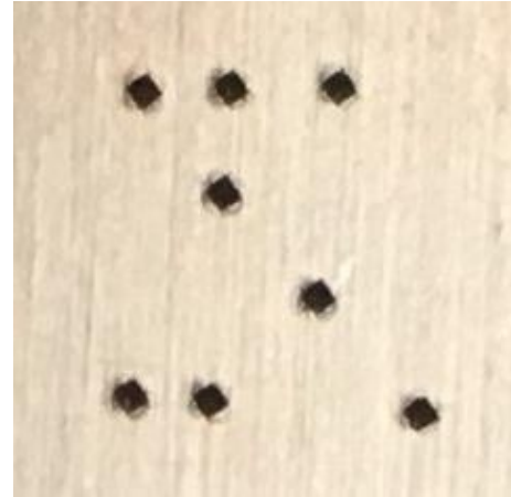
Figure 1: Hardness Indents in Copper from PHT-6005, with eight indents being made in a 4 x 4 grid area.
