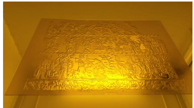
Figure 4. Photopolymer plate after exposure and washing-off, in the final stage of curing.
