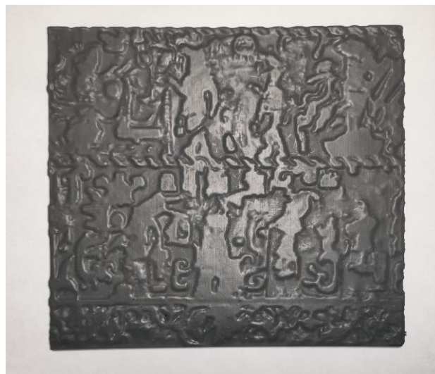
Figure 8. Surface relief printed by stereolithography
