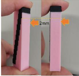
**Figure 6.** At the embedding depth of 2 mm, the FSC is completely hidden. So we can embed the FSC 2 mm deep and get clear information reading.
