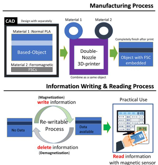
Figure 1. The workflow of the process of manufacturing 3D object with an embedded FSC and the process of information recording in practical use.
