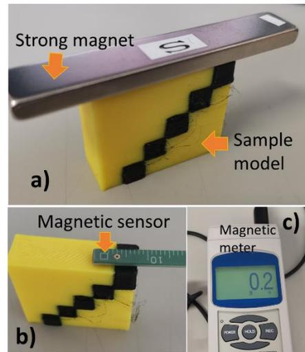
**Figure 2.** Steps of experiment methodology: a) place the strong magnet on the sample, b) measure the magnetic flux by placing a magnetic sensor on the surface of the sample, c) read the magnetic flux and polarity.
