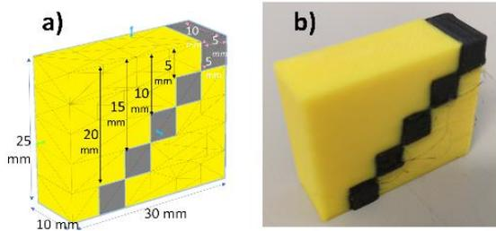
**Figure 3.** Sample1: a) design, and b) real 3D model. The yellow color is PLA and the black color area are the ferromagnetic storage cells (FSCs) printed as ferromagnetic filaments. Each FSC had been embedded at a depth different by 5 mm (totally, 5 positions).
