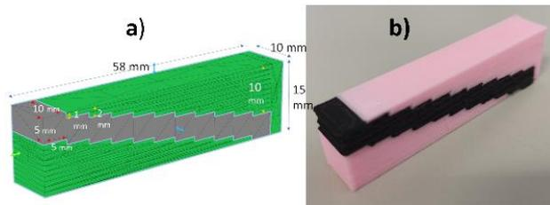
**Figure 4.** Sample2: a) design, and b) real 3D model. The pink color is PLA and the black color is FSC. Each FSC has embedded depth different in 1 mm, totally 11 positions
