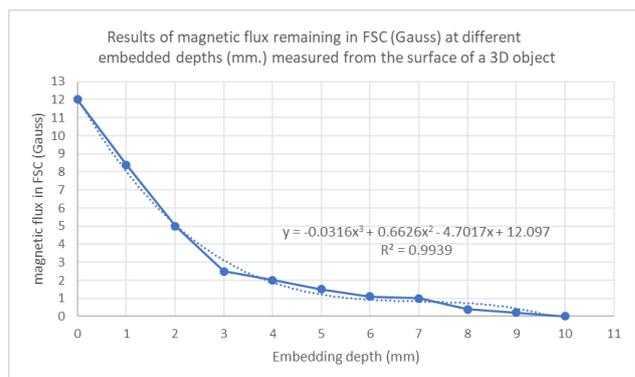
**Figure 5.** Results of magnetic flux remaining in FSC (Gauss) in different embedding depth (mm) measured from the surface of a 3D object
