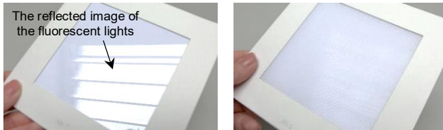
Figure 1. Examples of samples when the evaluation for defining standard samples was performed. Left: The mirror finished acrylic board whose image-perceptibility was defined as 100. Right: An example of another sample.
