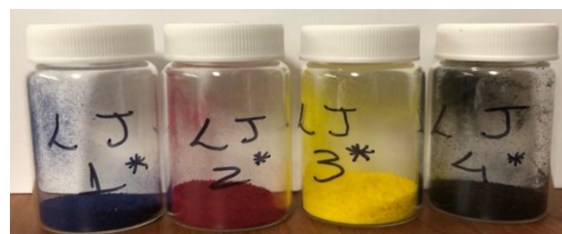
Figure 1. Vial with the CMYK laserjet inks after been dried and milled.
