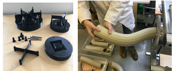
Figure 5. Smart Tooling for Ceramic Extrusion, Tavs Jorgensen
