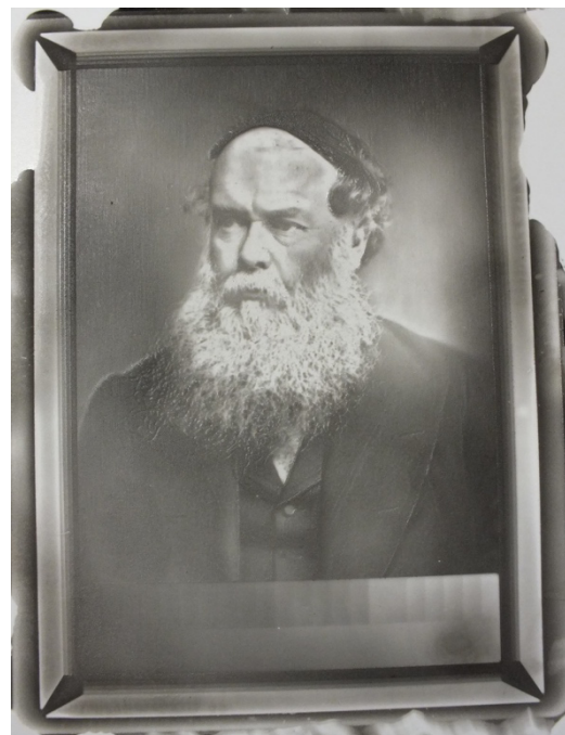
Figure 1. An example of a Woodburytype, printed using a standard silicone mold of a CNC milled plate. This displays all the range, print height difference and weaknesses of a generic Woodburytype print.
