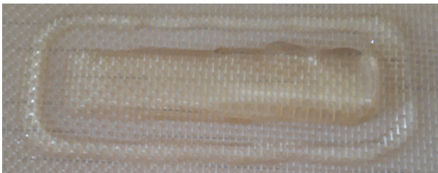
Figure 6. Example of the direct gelatine printing of the step-wedge image from Fig. 2. Above shows how the material is fed to the nozzle and subsequently the substrate. The ink contains no pigment so that the overall structure is more obvious. Below is the final set film, showing how the step-wedge becomes a smooth incline and the standard defects in this process, including the loss of resolution and uneven edges. However, the information of a increasingly thicker film is
