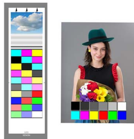
Figure 1. Images for xenon light exposure testing; (left) 30 patches for measurements, (right) Pictorial image for visual assessments
