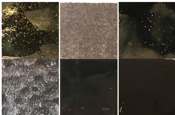
Figure 6. ANP silver nanoparticle ink (IJ4) on different substrates. On top from left Paper 1, Paper 2 and Paper 3. On bottom from left Paper 4, Paper 5 and PET.
