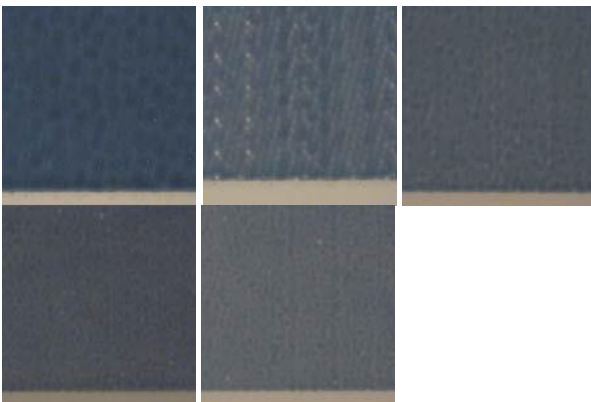
Figure 10. Rotary screen printed PEDOT layers (Screen 1) on Paper 4 substrate using different screen types. On top from left 125W, 125V and 215V. On bottom from left 305S and 305V.
