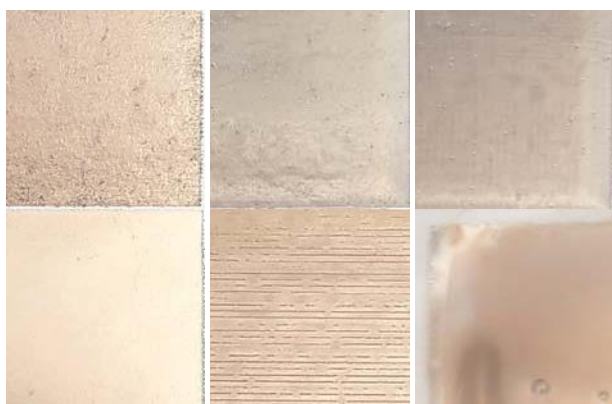
Figure 5. Orgacon silver nanoparticle ink (IJ3) on different plasma treated substrates. On top from left Paper1, Paper 2 and Paper 3. On bottom from left Paper 4, Paper 5 and PET.
