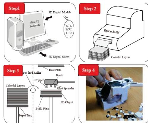
**Figure 1. Traditional paper-based 3D printing process workflow (Four steps)**
