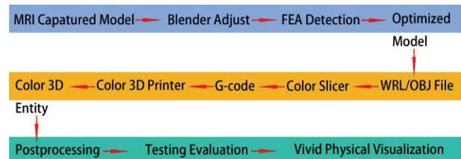
**Figure2. Proposed integrated paper-based 3D printing process workflow**
