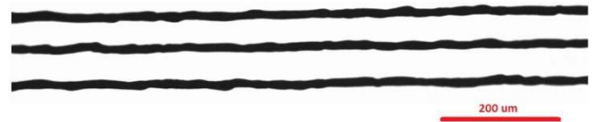
Figure 9. Batch of fibers with fluctuating morphology. Mean Batch Diameter: 11.93 +/- 0.58 \mu\text{m} Mean Batch UTS: 0.64 +/- 0.44 GPa
