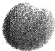
Figure 6. A microphotograph of laser speckle pattern generated on the surface of an ink droplet
