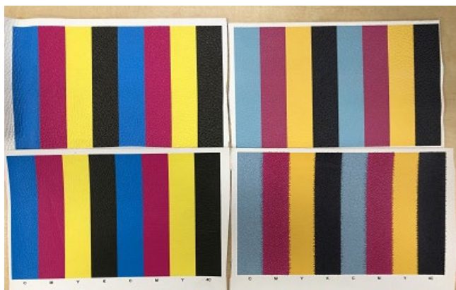
Figure 3. Image formed on leather (upper left; UV ink (product A) on the natural leather, upper right; Dye ink (product B) on the natural leather, lower left; UV ink on the synthetic leather, lower right; Dye-ink on the synthetic leather)
