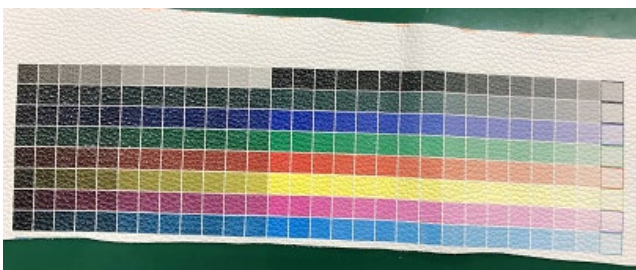
Figure 6. Images formed with ink A (aqueous resin ink)
