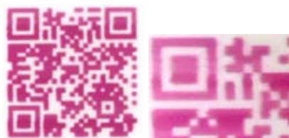
Figure 7. QR code with 0.75 mm cell size printed with the reversible photochromic ink (ink 3) on photo paper. Pictures are taken with a camera (left) and a with a mobile phone microscope (right).
