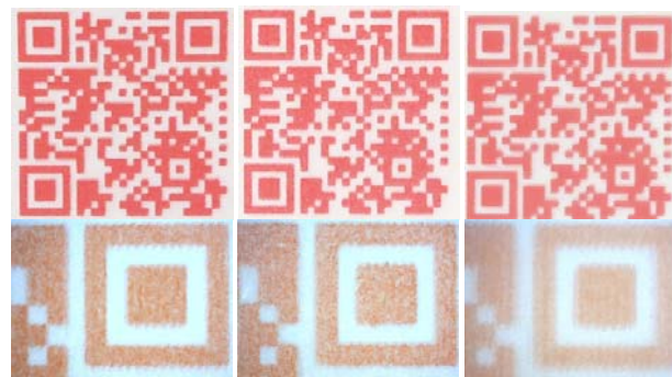
Figure 3. QR codes with 0.75 mm cell size printed with the thermochromic ink (ink 1) on different substrates: from left copy paper, label and photo paper. Pictures are taken with a camera (above) and with microscope (below).
