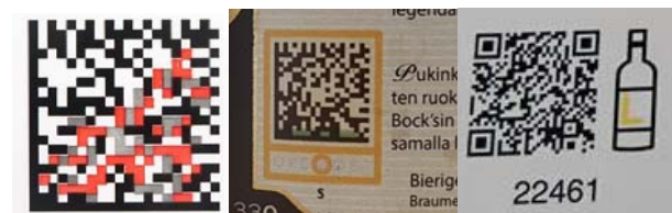
Figure 1. Options for using functional inks as part of QR codes. From left: (red and grey) cells printed with functional inks, (green) area printed at the bottom of the code with functional ink, and OCR (yellow letter "L") combined with QR codes.
