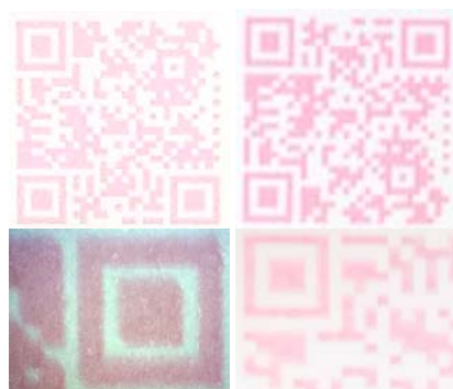
Figure 5. QR codes with 0.75 mm cell size printed with the irreversible photochromic ink (ink 2) on label (left) and photo paper (right). Pictures are taken with a camera (above) and with microscope (below).
