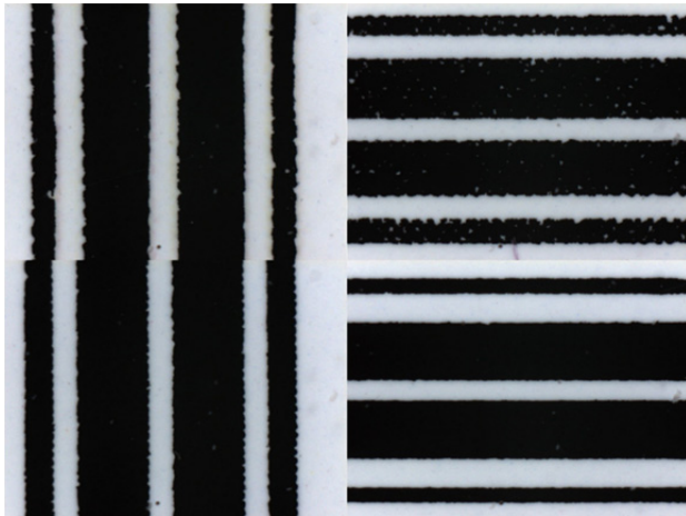
Figure 3. Horizontal and vertical barcode resin transfer at 300 dpi (top) and 600 dpi (bottom), 12x magnification.
