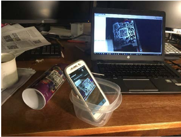
Figure 4. Example of imaging setup using the proposed approach. The notebook has loaded a web-based application to drive an imaging device, which in this case is the phone in the scene. The video feed from the phone, viewable on the phone screen, is processed on the notebook as if the video was obtained from a computer peripheral.
