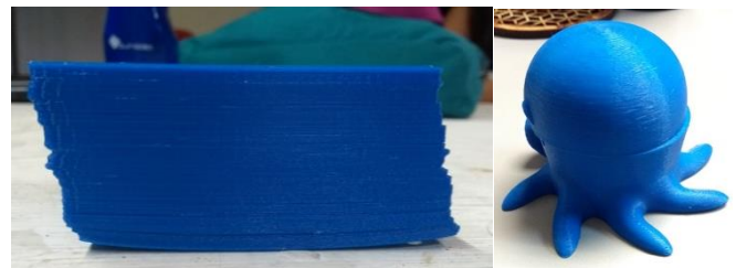
Figure 1 Displacement of layers in the printing process
