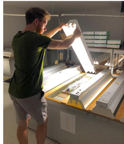
Figure 3. Charles Wilhelm removes a 3D color target from an accelerated fluorescent test unit.
