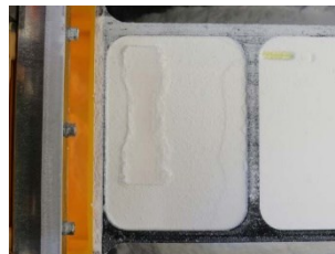
Figure 9. Dog bone being printed, resolution of 2500 dpi in X and 600 dpi in Y, no deposition pattern, 10 th layer
