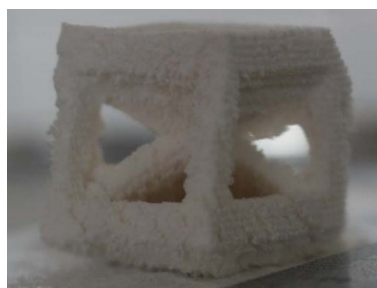
Figure 2. Lattice cube, resolution of 2500 dpi in X and 600 dpi in Y, layer thickness of 0.25 mm, deposition pattern x4
