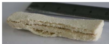
Figure 3. Dog bone presenting delamination, resolution of 2500 dpi in X and 400 dpi in Y, layer thickness of 250 \mu\text{m} , deposition pattern x4
