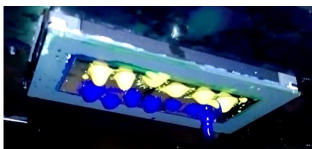
Figure 3. Nozzle plate surface after purging
