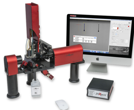
Figure 2. Example test setup, with JetXpert dropwatcher, Dimatix Samba printhead, and GIS drive electronics
