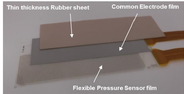
Figure 9. Structure of Flexible Pressure Sensor
