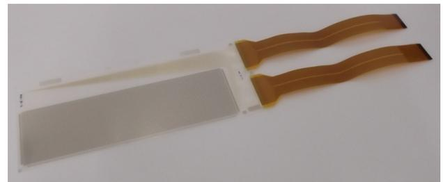
Figure 6. Flexible pressure sensor with 1.2 mm pitch, 5760 pixels (sensor area is 4.8 cm x 17.3 cm)
