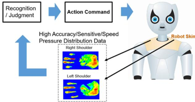
Figure 7. Robotic skin tactile identification system
