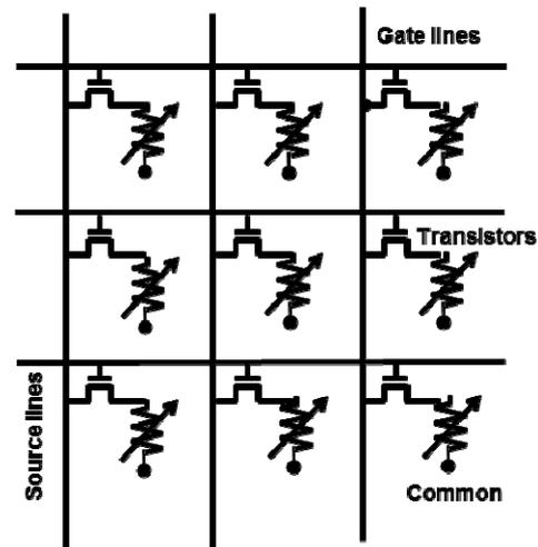
Figure 5. Equivalent circuit of pressure sensitive sensor
