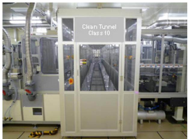
Figure 2. Clean tunnel connected printers and curing funnels
