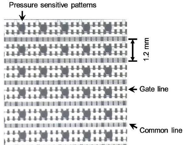
Figure 4. Surface view of pressure sensor elements.
