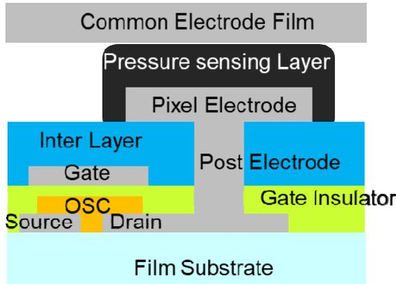
Figure 3. Cross sectional view of pressure sensor with the top gate structure
