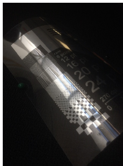
Figure 4: a packaging ink displaying a true metallic effect printed by Vista onto plastic sheet (D50~5µm aluminium flakes).
