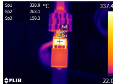
Figure 8 Thermograph of new 3D hotend
