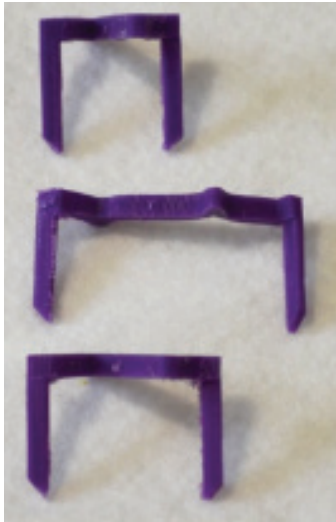
Fig. 4. Biodegradable PLA staple with self-tightening function. Top: as printed shape; middle: after programming; bottom: after heating for shape recovery
