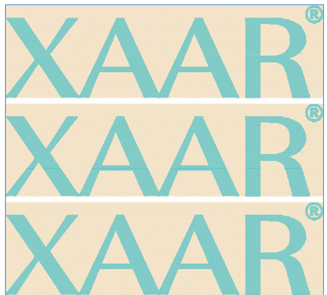
Figure 8. Example of a mechanically misaligned system. -10\ \mu\text{m} at the top, and +10\ \mu\text{m} in the center and at the bottom. The bottom text corrected by software using the vernier software alignment. This image is magnified 5 times.
