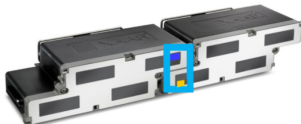
Figure 2. As in Figure 1 for actuators inside a printhead, the vernier arrangement works for actuators in adjacent printheads. A vernier design, as implemented in the Xaar 5601 GS3 printhead guarantees that 2 nozzles will be aligned inside the overlapping region to within 1 \mu\text{m}
