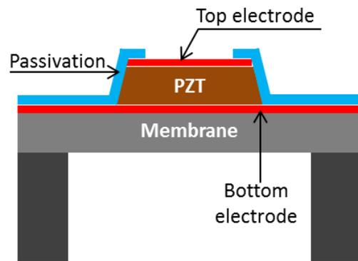
Figure 1. Schematic representation of the cross-section of the actuator.
