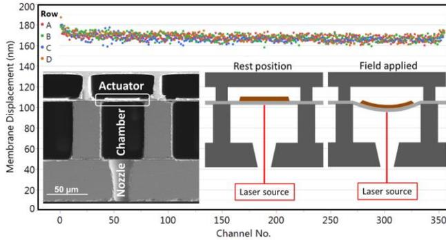
**Figure 2.** Example of measurements of the membrane displacement by channel number using AixACCT's TNT tool. Measured at 100 kV/cm, over 1420 channels total. The insert shows the cross section of a single actuator, including chamber and nozzle, and schematic of displacement measurements by 5  $\mu$ m laser beam through the nozzle.
