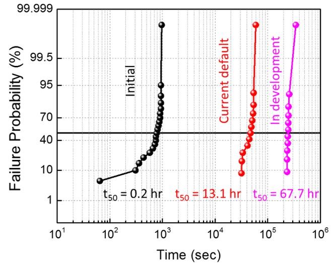
**Figure 4.** Comparison of the failure probability vs. time for sol-gel PZT films on different stages of development. Test performed at 200°C and applied DC field of 300 kV/cm.
