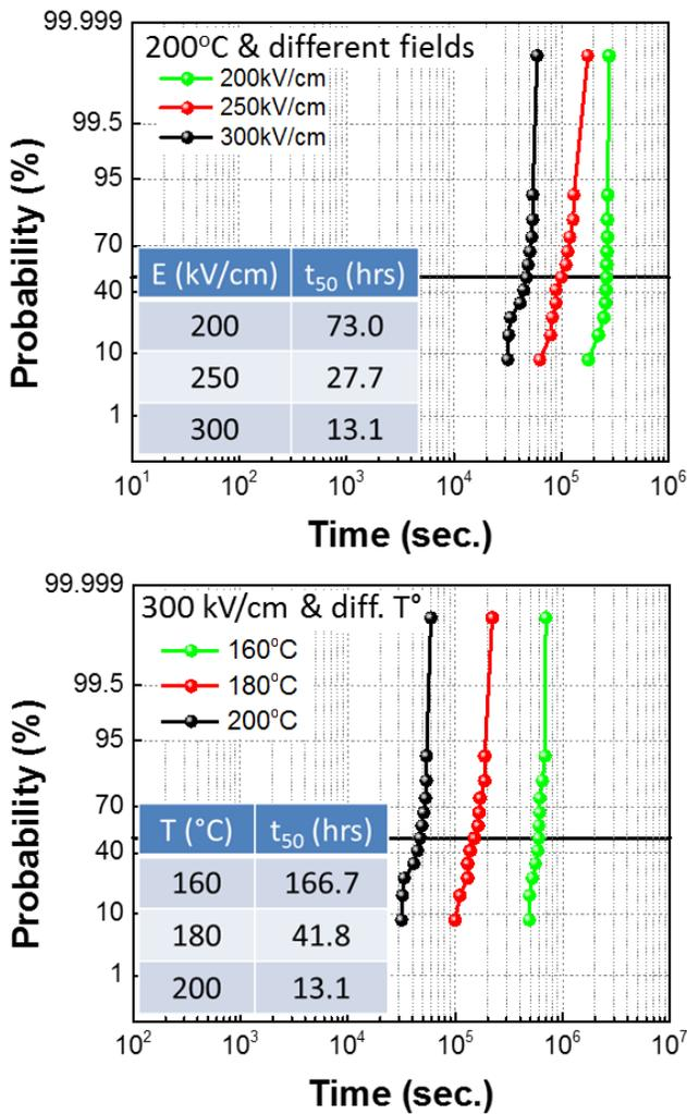
Figure 5. HALT data at constant temperature for different fields and at constant field at different temperatures of “current default” sol-gel PZT thin films.
