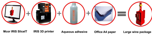
Figure 1. From the left to right, the pics are Mcor IRIS SliceIT, IRIS 3D printer, Aqueous adhesive and Office A4 paper, printed wine package model respectively.
