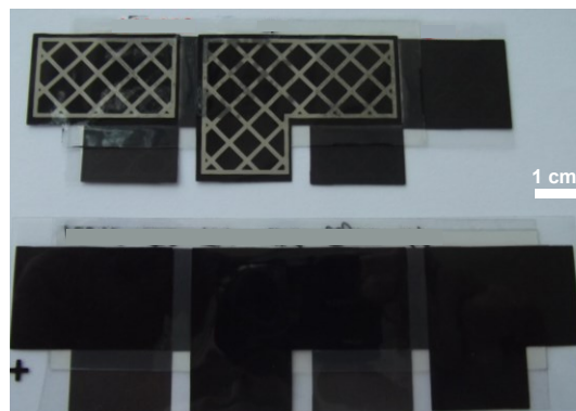
Figure 7. Printed batteries up) with and down) without silver grid. The upper battery contains three cells, the lower four. © Fraunhofer ENAS
