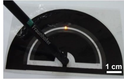
Figure 9. Inlay of a greeting card, driving an orange LED by two curved batteries. The printed push button is pressed by a pencil. © Fraunhofer ENAS
