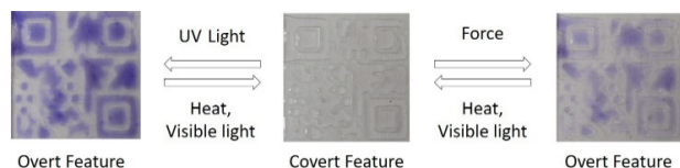
Figure 11: Transformation pathways of a printed SP-PDMS QR code.
