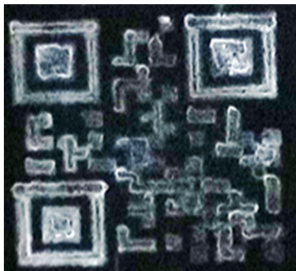
Figure 8: QR code security mark printed using an M3D aerosol jet printer after wiping with an aqueous solution containing a colored ink.
