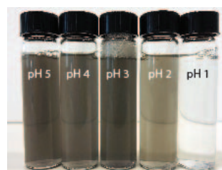
Figure 4. Images of the dispersions centrifuged at 500 rpm at concentrations ranging from pH 1 to 5
