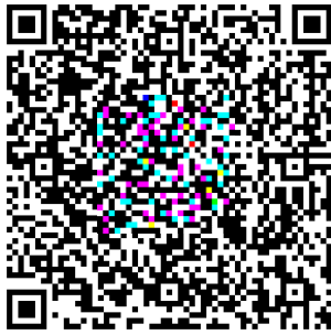
Figure 7. Example QR-Data Matrix hybridization where quiet zones and finder patterns have been removed entirely. In this case, the static data associated with the black & white Data Matrix is also no longer readable by standard barcode readers, but would be if the quiet zones and finder patterns were superimposed over the QR code around the edges of the color region.
