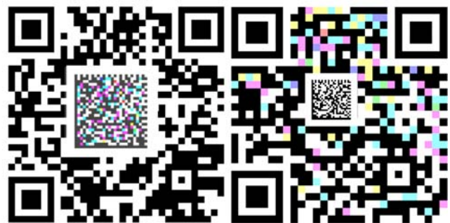
Figure 6. Comparison of different hybrid QR/progressive Data Matrix codes; the progressive portion is the same in both examples. Note that it is possible to represent nearly arbitrary graphical content within a QR code without significantly disrupting the quality of the payload [6]. Left side contains 3 channels of information: 1-black & white QR code, 2-black & white Data Matrix, 3-color channel in the Data Matrix. Right side also contains 3 channels of information, however, in this case the color channel is associated with the QR code rather than the Data Matrix barcode.
