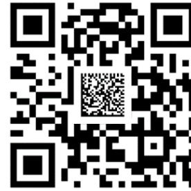
Figure 5. Example hybrid code: a Data Matrix code contained within a QR code. By scanning the design at different distances, both codes are readable with standard tools.
