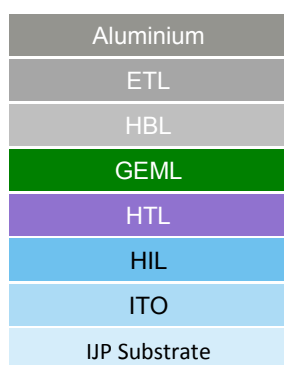
Figure 1. Printed OLED Device Architecture. HIL, HTL and GEML are inkjet printed. HBL, ETL and Cathode are deposited via vapour deposition
