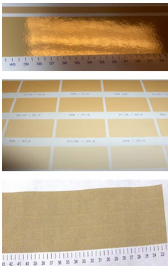
Figure 6. Impact of media pore size on visual appearance of the MeOx print. The same \text{Fe}_3\text{O}_4 nano-particles formulation was printed on: (top) high end photopaper - complete retention of MeOx on media surface; (middle) brochure paper – partial penetration of MeOx into media pores; (bottom) plain office paper – full penetration of MeOx particles inside the media.
