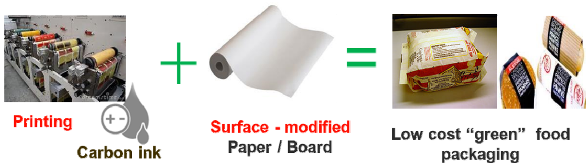
Fig. 1 100% paper-based and using standard printing to add a conductive layer to improve performance & lower cost
