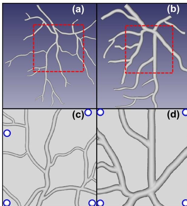
**Figure 2** (a) The arterial and (b) venous vasculature of human placenta and corresponding moulds (c) for artery and (d) vein designed in FreeCAD. Red squares show the region of interest. Blue circles correspond to holes in the moulds used for screws to fix two halves of the mould together.
