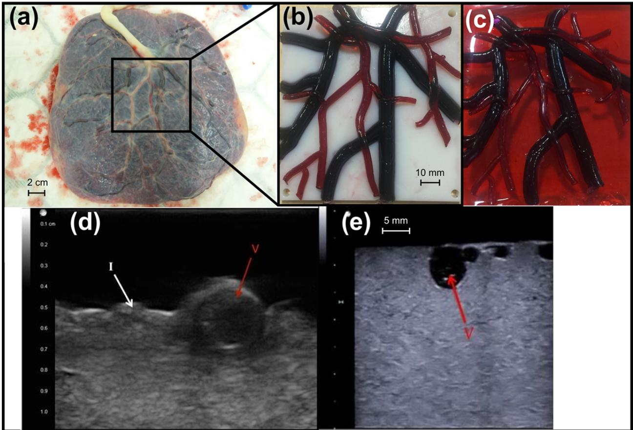
**Figure 3** (a) A photograph of human placenta, (b) 3D printed moulds with the gelwax vasculature of human placenta, (c) an ultrasound image of the phantom, (d) an ultrasound image of the human placenta and (e) of the imaging phantom. The placenta (d) shows some indentation (I) on surface and the vein (V) is slightly less embedded than that shown illustrated by the phantom (e). The surface of the placenta modelled in the phantom is smooth.
