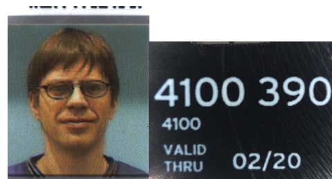
Figure 8. UV inkjet is used to print photographs and account information on financial cards.
