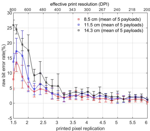
**Figure 11.** Average raw bit error rate for printer C1200 across 5 payloads at video capture distances of 8.5, 11.5, and 14.3 cm.
