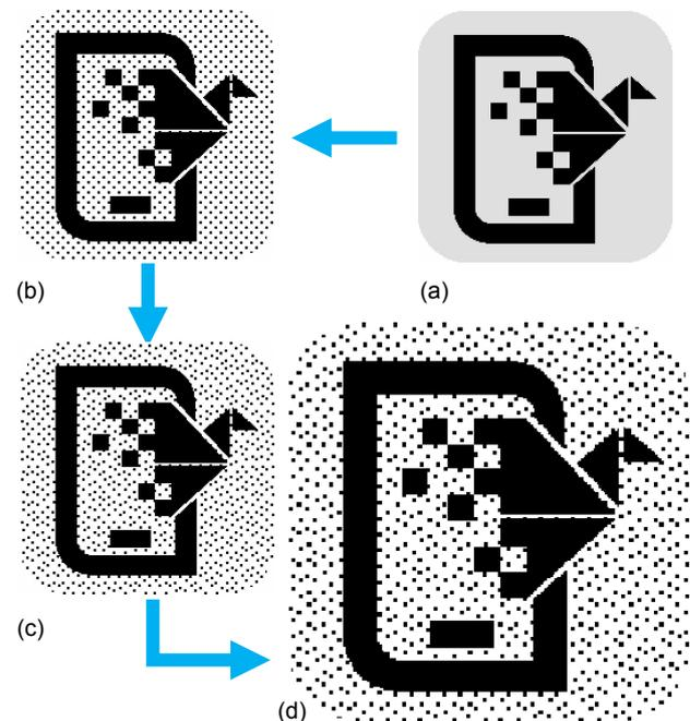
Figure 2. Steganone generation and printing. (a) Gray scale input image, (b) Clustered-dot halftone, (c) Steganone, and (d) Scaled by 1.6x when printed.
