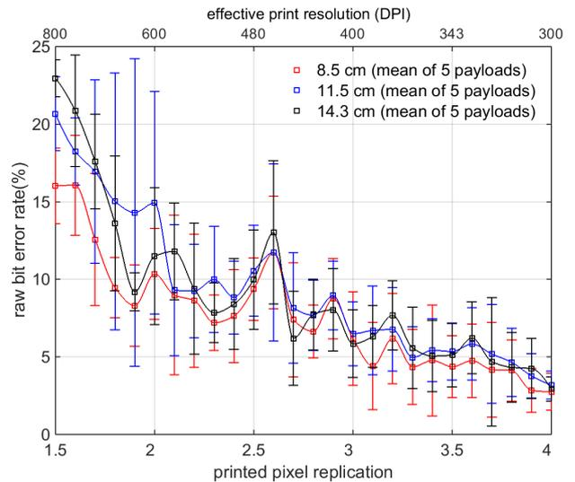
**Figure 12.** Average raw bit error rate for printer D1200 across 5 payloads at video capture distances of 8.5, 11.5, and 14.3 cm.
