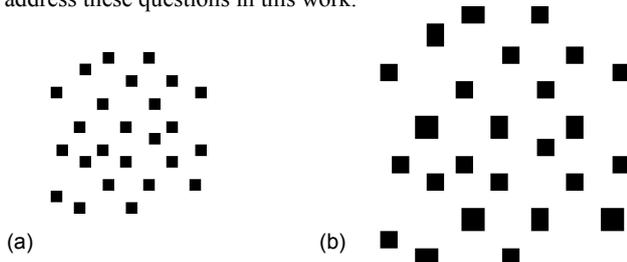
Figure 3. Nearest-neighbor scaling of an array of 2x2 clusters by 1.6x.
