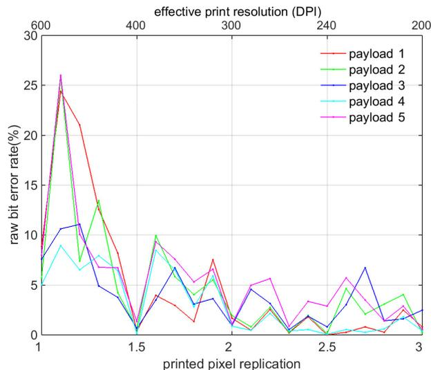
**Figure 7.** Raw bit error rate for printer A600, captured at 8.5 cm for 5 different payloads.
