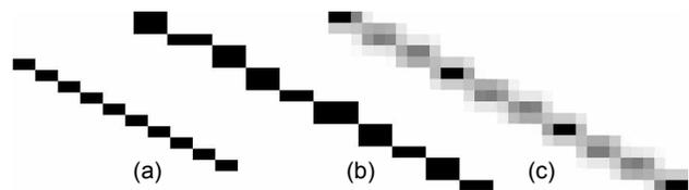
Figure 1. Scaling a one-pixel wide line by 1.6x. (a) Input, (b) Nearest-neighbor scaling, (c) Bilinear scaling.
