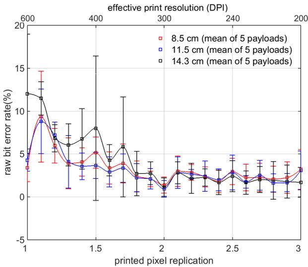
**Figure 10.** Average raw bit error rate for printer B600 across 5 payloads at video capture distances of 8.5, 11.5, and 14.3 cm.
