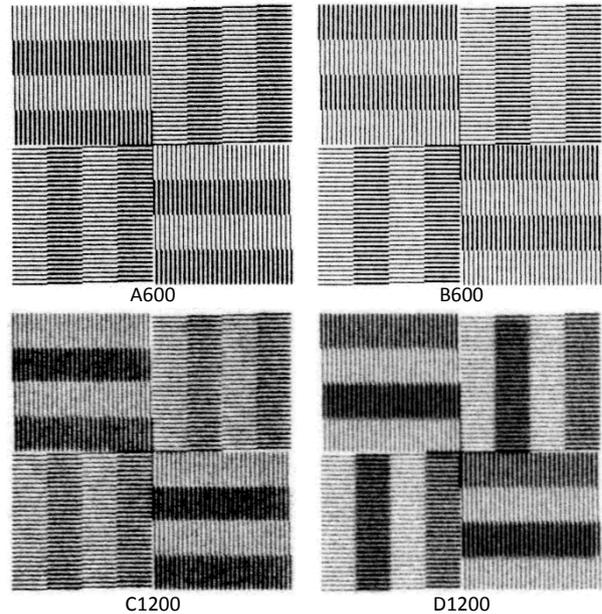
Figure 5. Results of scaling by 1.5x. Output from 4 different printers.
