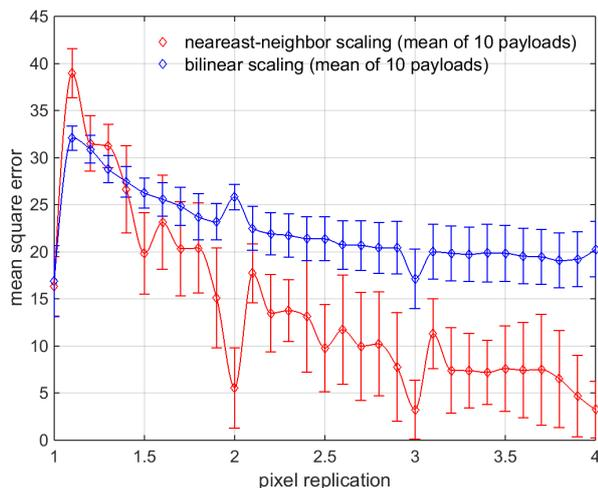
**Figure 18.** Average MSE for the bird image with 10 different payloads for a digitally simulated printer that pixel replicates by nearest-neighbor and bilinear scaling.
