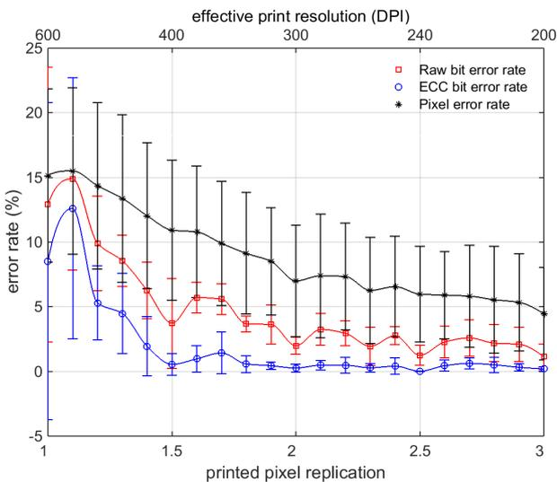
Figure 16. Average raw bit error rate, ECC error rate, and pixel error rate for 4 different source images for printer A600 across 5 payloads at a video capture distance of 8.5 cm.
