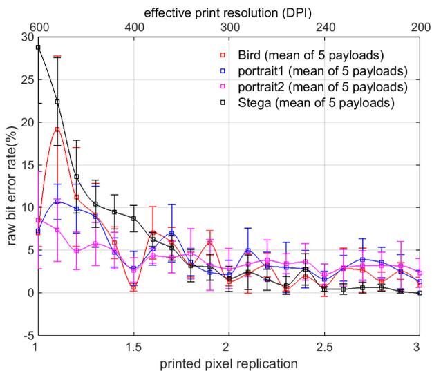
Figure 15. Average raw bit error rate for 4 different source images for printer A600 across 5 payloads at a video capture distance of 8.5 cm.
