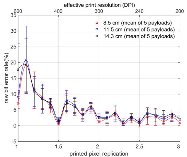
**Figure 9.** Average raw bit error rate for printer A600 across 5 payloads at video capture distances of 8.5, 11.5, and 14.3 cm.
