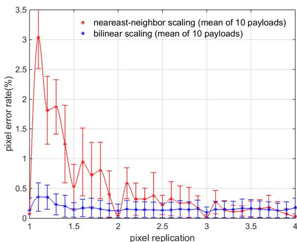
**Figure 19.** Average pixel error rate for the bird image with 10 different payloads for a digitally simulated printer that pixel replicates by nearest-neighbor and bilinear scaling.
