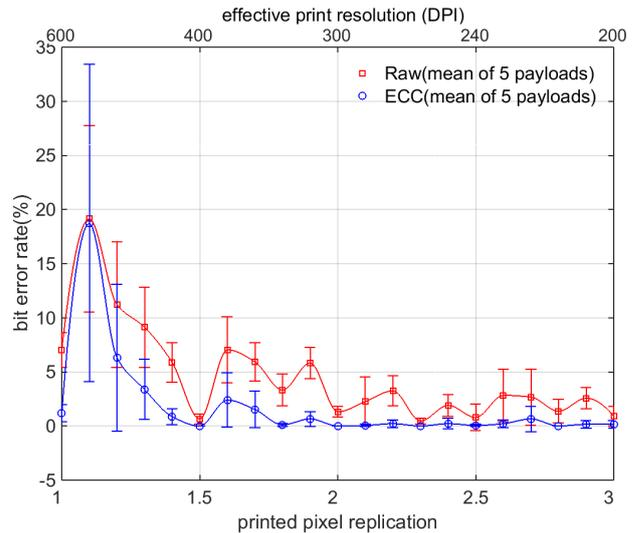
**Figure 8.** Average raw bit error rate and ECC error rate for printer A600, captured at 8.5 cm.
