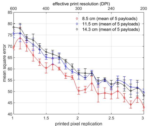
**Figure 13.** Average mean square error for printer A600 across 5 payloads at video capture distances of 8.5, 11.5, and 14.3 cm.
