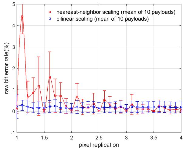
Figure 17. Average raw bit error rate for the bird image with 10 different payloads for a digitally simulated printer that pixel replicates by nearest-neighbor and bilinear scaling.
