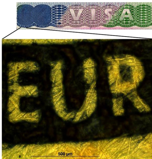
Figure 4 Intaglio print onto paper with microscope image
