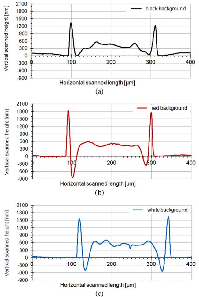
Figure 7. Surface profiles scanned over a single silver line after flashing with  $1.25 \text{ J/cm}^2$  without direct contact with the background: (a) black background; (b) red background; (c) white background.
