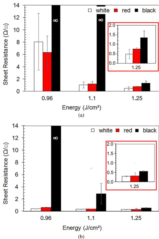
Figure 8. Measured sheet resistance of silver films in dependence on flashing energy and background: (a) with contact; (b) without contact.
