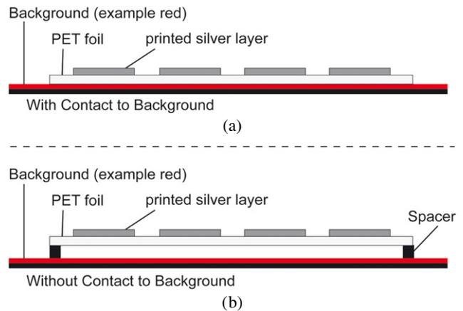
Figure 3. Graphical description of the experimental setup: (a) with direct contact with the colored background; (b) without direct contact with the colored background.
