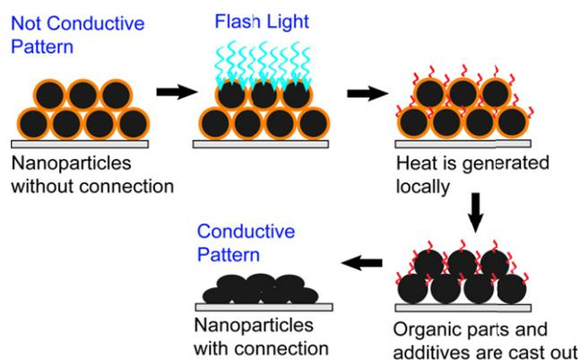
Figure 1. The basic process of IPL sintering of an NP metal layer.
