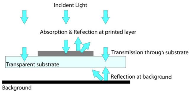
Figure 2. Graphical description of possible absorption and reflection schemes of a printed metal layer on a transparent substrate with 3 mm distance to a colored background.
