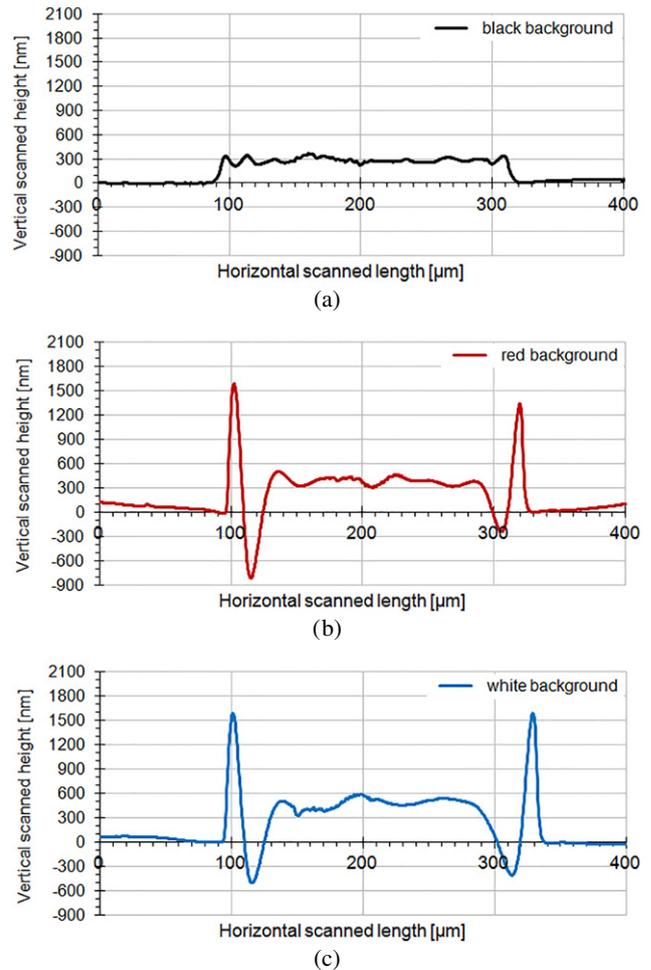
Figure 5. Surface profiles scanned over a single silver line after flashing with  $0.96 \text{ J/cm}^2$  without direct contact with the background: (a) black background; (b) red background; (c) white background.
