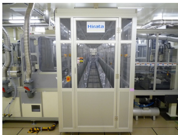
Figure 2. Clean tunnel connected printers and curing funnels
