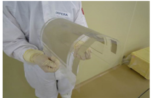
Figure 6. Printed sample of flexible and bendable TFT array film
