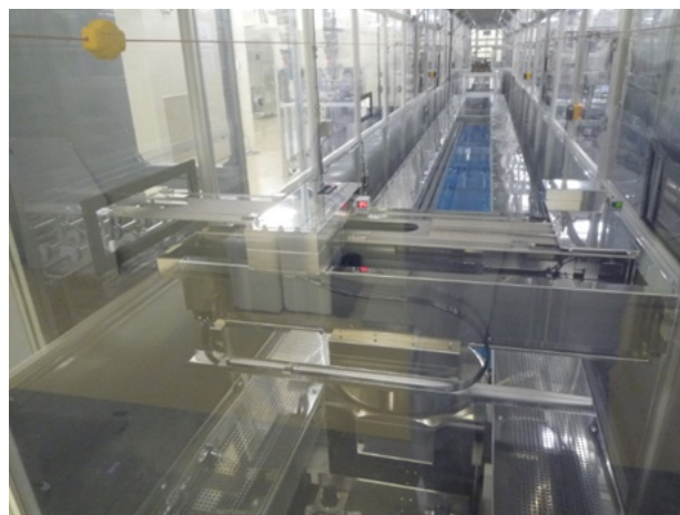
Figure 1. Substrate transporting robot in clean tunnel of automated print manufacturing line
