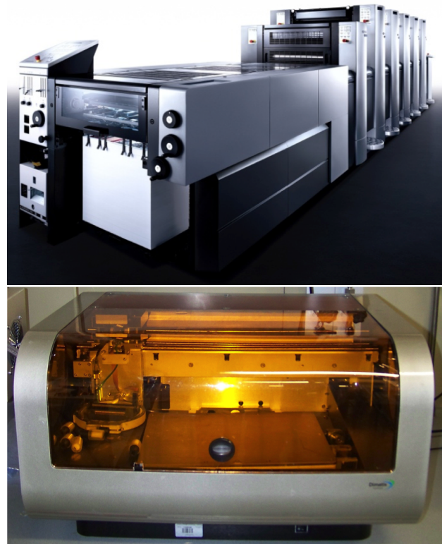
Figure 3. Printing devices used in this research project. Top: Heidelberg Speedmaster 52. Bottom: Dimatix DMP2831.
