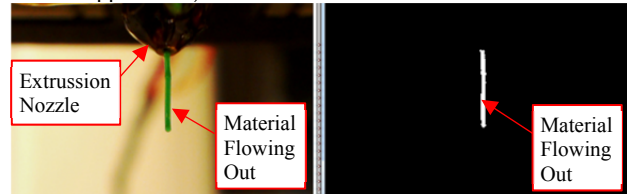
Figure 4. Example of binarization (Left: Original image, Right: Binarized image for green filament detection)
