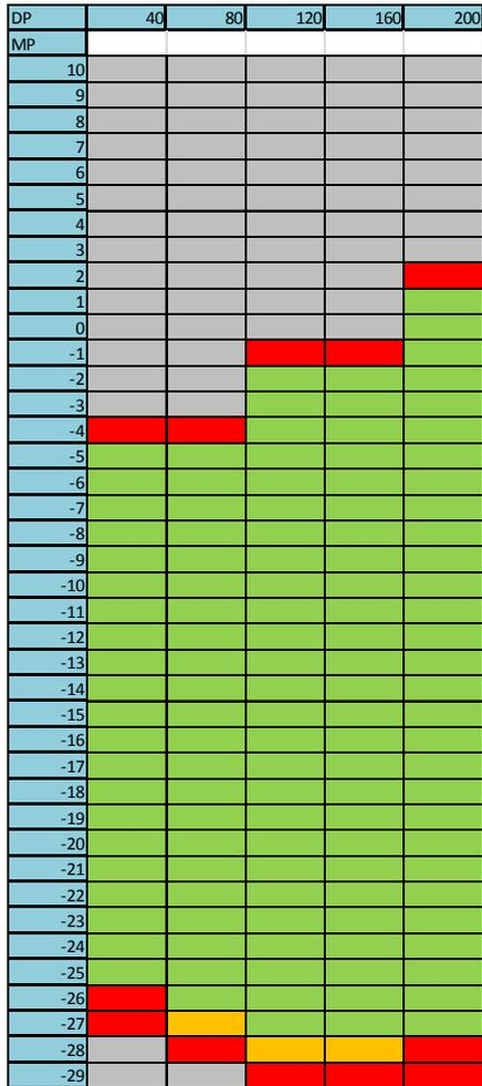
Figure 8 MP window results for SunJet ULX cyan, showing that the MP window (range of green cells) increases as DP increases.
