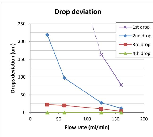
**Figure 4** Dot placement errors for the first 4 dots from the burst of 10 drops as function of the flow rate (30, 60, 125 and 160 ml/min). Idling time before the burst of 10 drops was 5 minutes.
