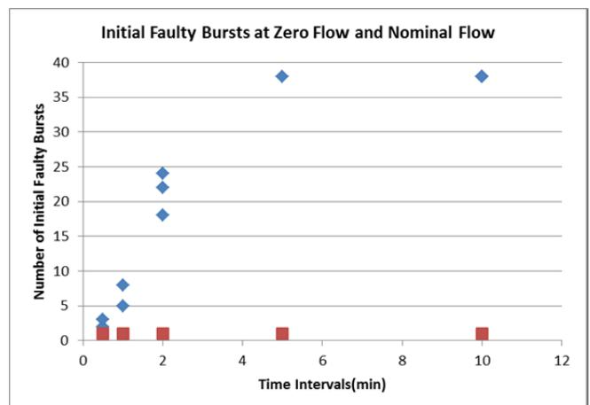
**Figure 6** The number of initial bursts with missing or strongly misplaced drops after different time intervals of zero flow, and 10 seconds after restarting of ink flow directly after the time intervals with zero flow.
