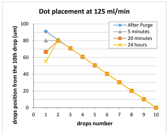
**Figure 5** At standard operation conditions the Xaar 1001 printhead is operated at a flow rate of 125 ml/min. In the present experiment this was achieved at a differential pressure of 100 mbar.
