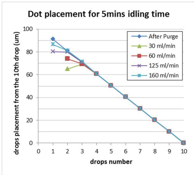
**Figure 3** Dot placement of the 10 dots from a burst in reference to position of the 10th and last dot in the burst. Printing at different flow rates with a constant 5 minutes idling time before firing each test run.
