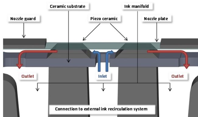
Figure 1 Schematic of Xaar TF Technology® showing the path of fluid into the piezoceramic channels, directly behind the nozzles, and out again.
