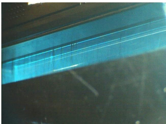
**Figure 7** Showing a good jetting 'curtain' (top) and unreliable, with some missing jets (bottom)
